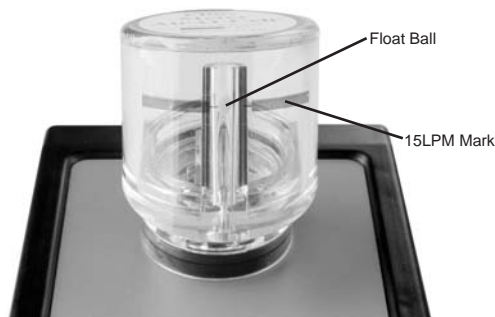
Adjust flow until ball is centered on line.
